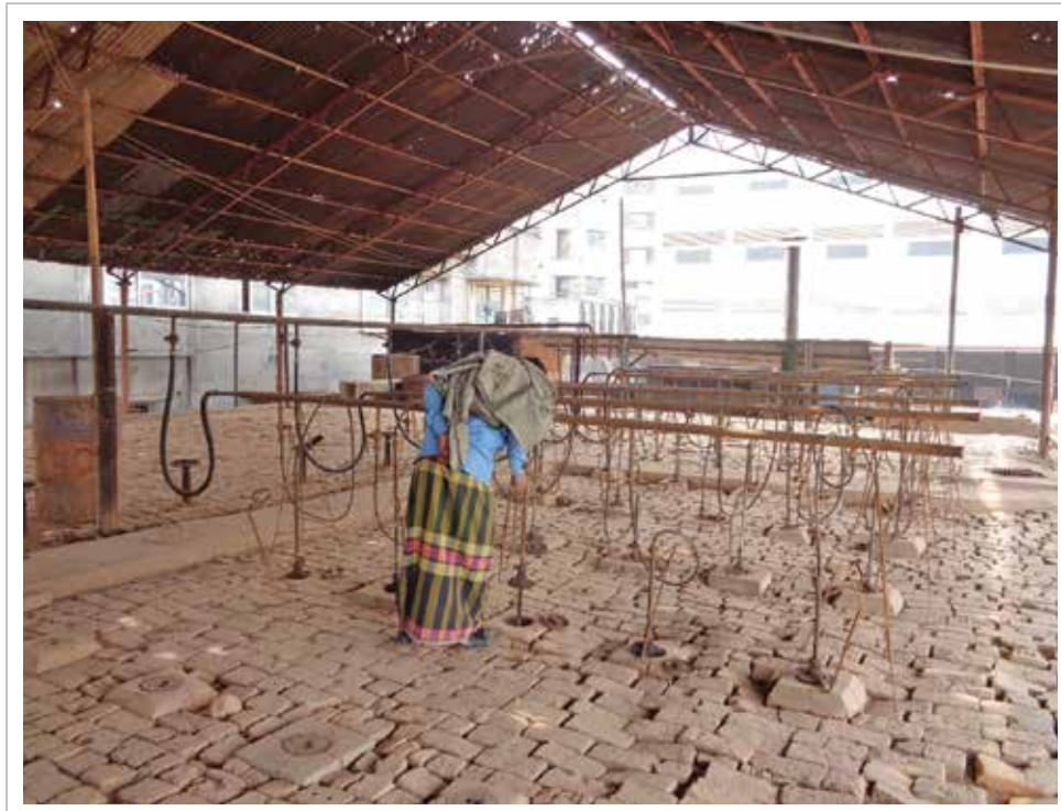
Figure 11: Use of Natural Gas in a Hoffmann Kiln in Bangladesh
