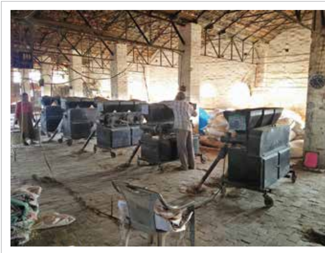
Figure 9: An octopus type coal feeder consisting of a coal crusher and delivery unit 19
