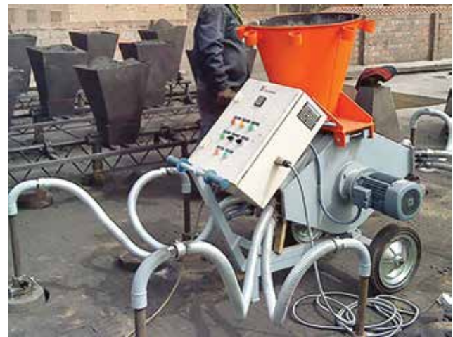
Figure 10: Trickle feeder for feeding biomass fuel in a Hoffmann kiln (Balaghat)
