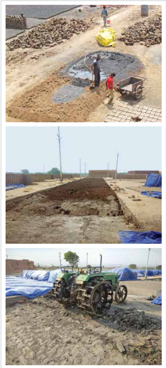
Figure 7: Mixing of fly ash with clay (Maharashtra & Telangana)
