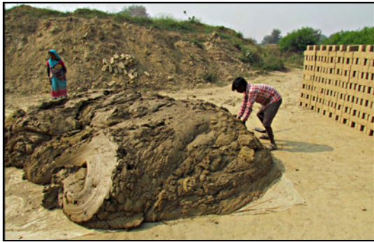
Figure 2.1: Clay-mixture must be kept on a plastic sheet
