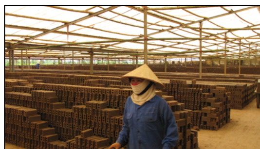
Figure 3.7: Drying of bricks under the shed
