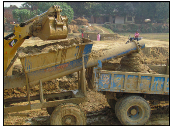
Figure 1.7: Clay-mixture prepared by Pug-mill machine
