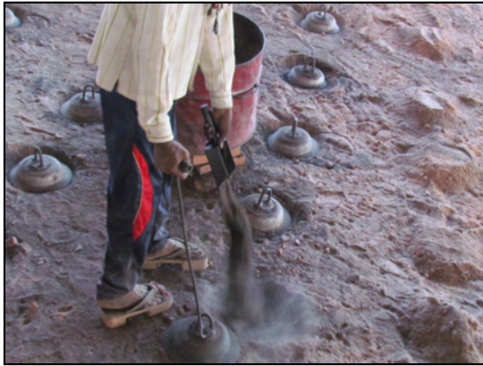
Figure 5.3: Small hand-shovel must be used to feed crushed coal
