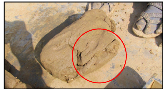
Figure 2.3: Formation of joint in the clot
