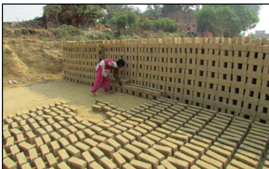
Figure 3.2: Drying bricks in hacks
