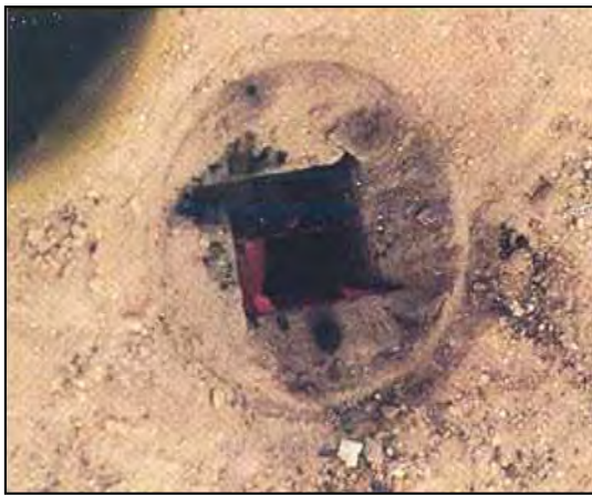
Figure 5.10: Insufficient temperature to burn the coal
