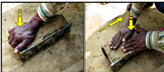
Figure 2.6: Correct way to press the clot into the mould
