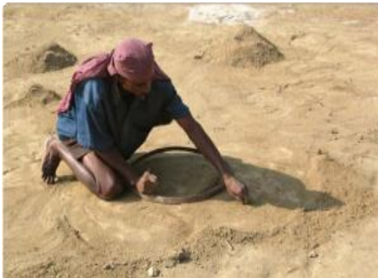
Figure 48: Preparation of moulding area 23
