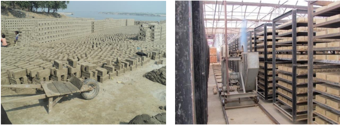
Figure 10: Natural and artificial drying of bricks
