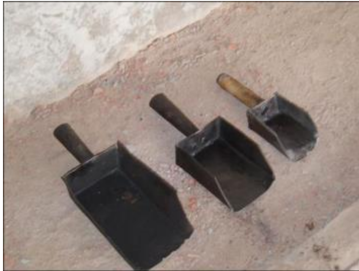
Figure 92: Different sized spoons are used in a Zig-zag kiln
