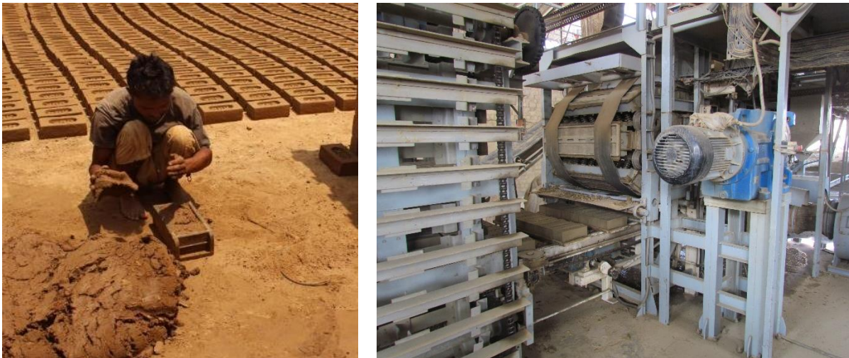
Figure 9: Manual and mechanized moulding of soft-mud bricks
