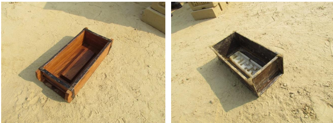
Figure 45: Types of moulds: Wooden Mould and metallic mould
