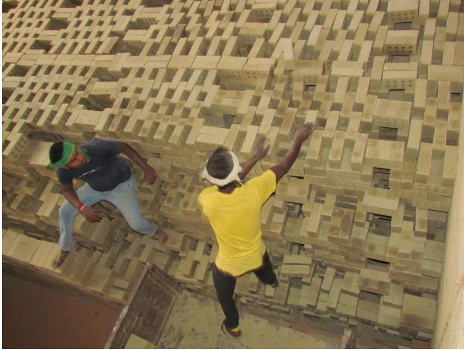
Figure 29: Stacking of green bricks
