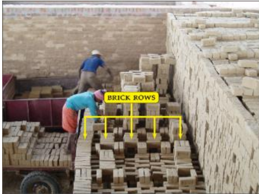
Figure 85: Brick-setting showing Jodi and Bandhan in a Zig-zag kiln
