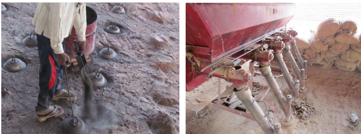
Figure 11: Hand-fed and stoker-fed firing of brick kiln
