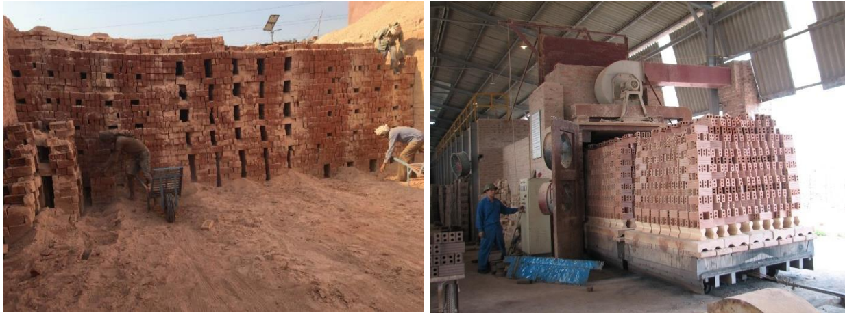
Figure 12: Fired bricks in the kiln
